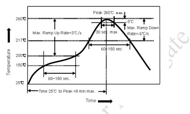
\*Above reflow soldering curve is from J-STD-020D.
